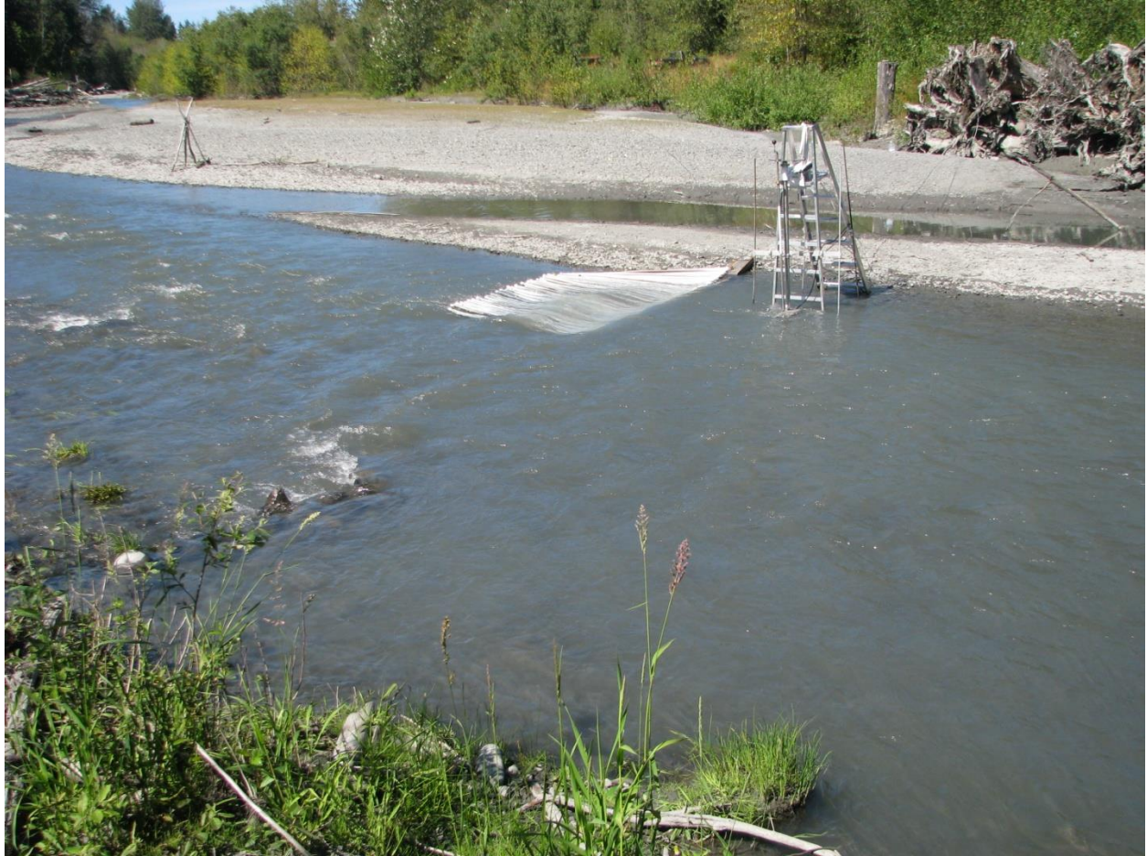
Figure 4. Old Mainstem SONAR site. The SONAR itself is attached to the pole mount which is in turn attached to the ladder. The PVC picket weir immediately downstream from the ladder directs fish away from the bank so they pass at least 5 m from the SONAR head.
